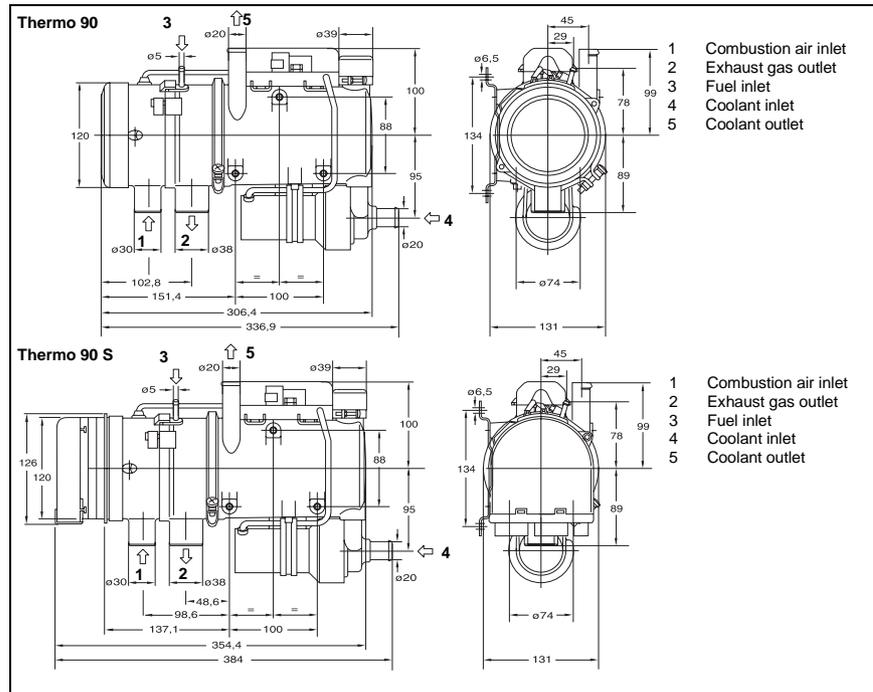
Fig. 2: Dimensions of the Heater
