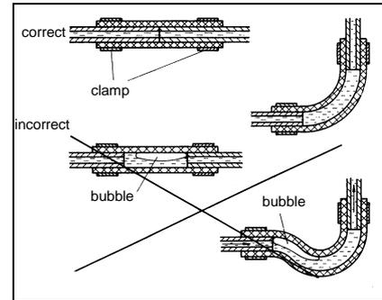
**Fig. 9: Pipe/Hose Connection**
