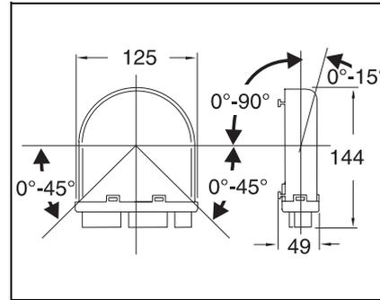
**Fig. 15: Control Unit T 90 S (from 03/97), Installation Position**
