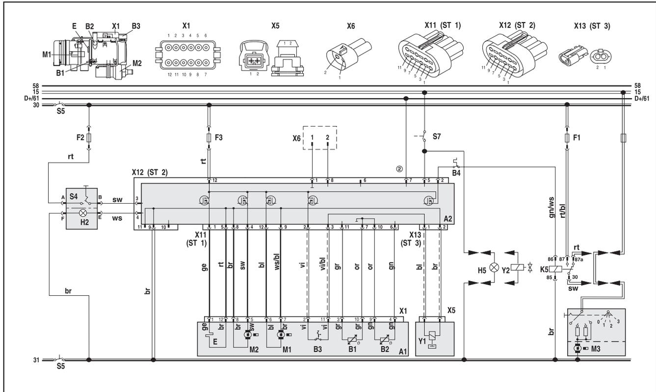
Fig. 20: System Diagram Thermo 90 S - ADR, 24V, for legende refer to page 10 and 11
