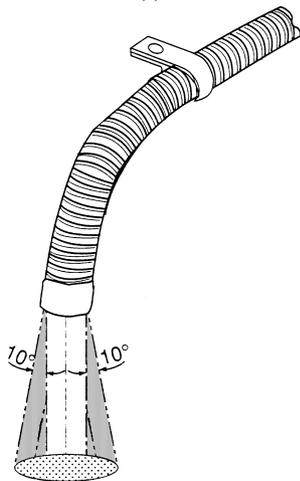
direction of discharge approximately vertical  $90^\circ \pm 10^\circ$
